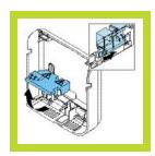
**2.** Open the safety cover. Use a small flathead screwdriver to loosen the clip.
