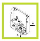
1. Pass the power supply cable through the opening on the back (A) or the cable entry point (B).
