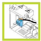
**4.** Connect the power supply cable to the screw terminals.
